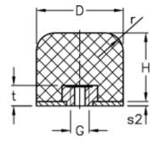
D = 125 t = 16 d2 = 4 G = M16 H = 100 Load capacity F (kN) = 150.0 Load capacity f (mm) = 55 Load capacity W (J) = 2240 r = 25.0
